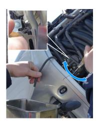
6. After draining, tighten the drain screw.
