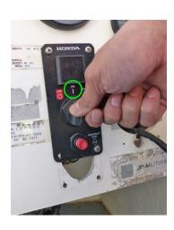
Turn the engine switch key to the ON position.
