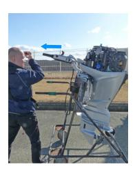
17. Pull the emergency starter rope several times to lubricate the inside of the cylinder. Then remove the emergency starter rope.
