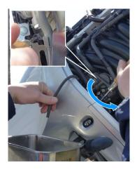
5. Drain the petrol into the drain pan as it flows out of the drain tube.
