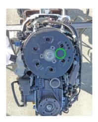
6. Set the ACG rotor so the cutouts are on the right and left sides of the ACG rotor as shown.
