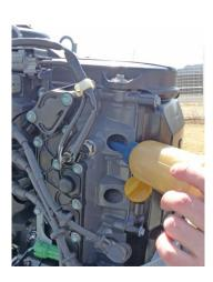
Pour a teaspoon of engine oil into all the spark plug holes.
