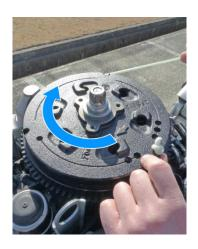
8. Wind the emergency starter rope clockwise 1 and half turns clockwise along the groove in the ACG rotor.
