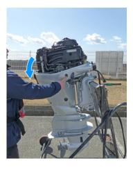
8. Tilt the outboard motor down.
